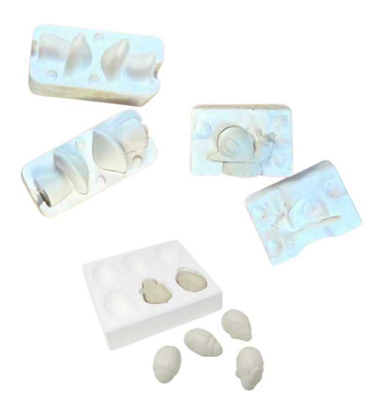
• Once removed Li-Qua-Che will be rigid but fragile. Handle the casting carefully.
